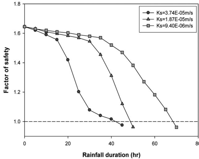
Fig. 1 FS (Factor of safety) of slope versus soil hydraulic conductivity (Ministry of Science, ICT and Future Planning of Korea 2013)
