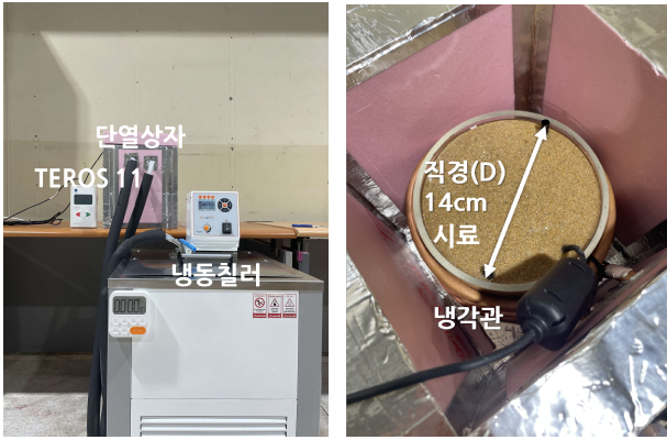
Fig. 1. Experimental setup for measurement of the unfrozen water content of sandy soil
