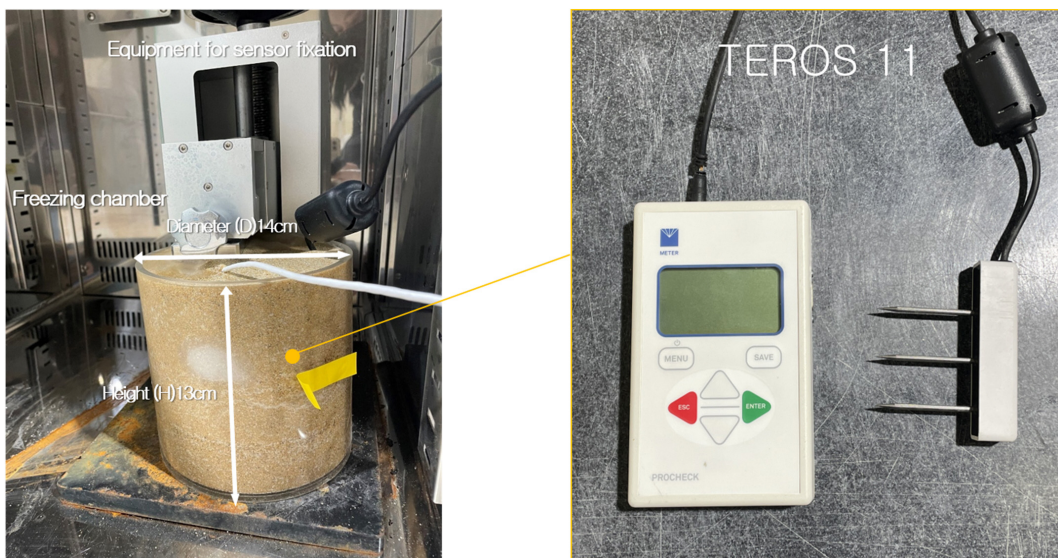
Fig. 6. Experimental setup for measurement of the unfrozen water content of frozen sandy soil
