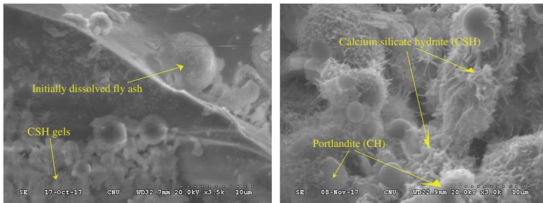
**Fig. 10.** SEM image of CLSM mixture made with cement.
